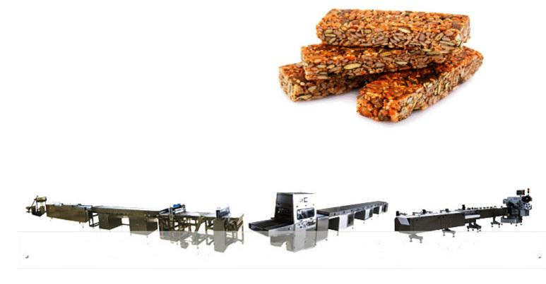
In addition, the Cereal Bar Production Line has a fully automated production method, using high-quafrequency converters to control the speed, and the production efficiency is guaranteed. The higher the per unit time, for the majority of manufacturers, it means that more orders can be received. Moreover, goods can be submitted within the specified time with quality and quantity.
