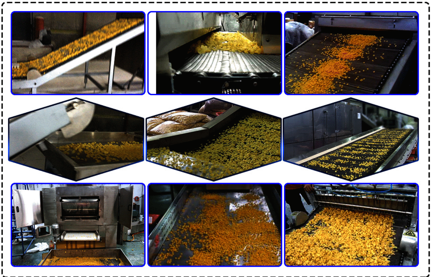
Site Picture of Corn Flakes Processing Line
