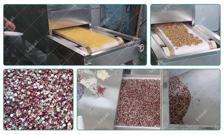
Test of Tunnel Microwave Drying Sterilizing Machine for Grain Millet Mung Beans Buckwheat Red Beans in Customer's Workshop
