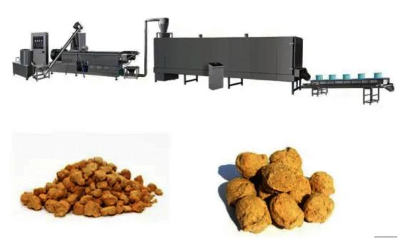
Soybean meat production line consists of mixer, screw conveyor, twin-screw extruder, airflow convey elevator, seasoning roller oil sprayer, cooler, packaging machine. The working conditions of the main equipment are as follows:
