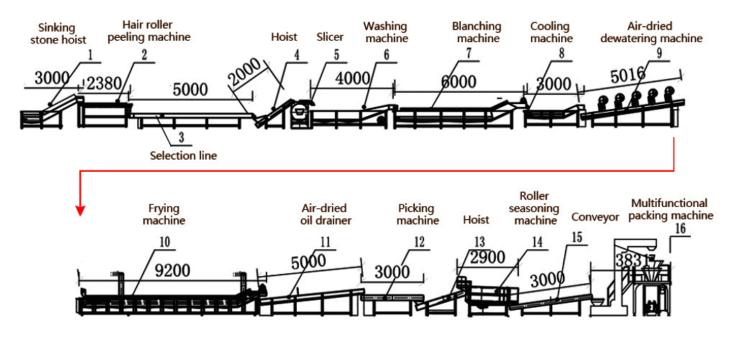
Flow Chart of Automatic Frozen French Fries Production Line Peeling -- Cutting -- Rinsing -- Blanching -- Shaken And Drained -- Frying -- Deoiling-- Seasoning --Freezing -- Weighing and Packing.Flow Chart of Automatic Frozen Fren
