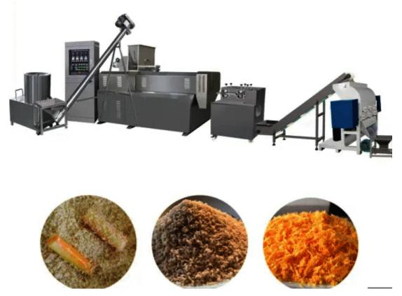
The bread crumbs production line overcomes the shortcomings of the previous equipment. It is design more reasonably, solving the difficult problems of the existing domestic equipment such as sticky matter the press rollers, low yield and forming rate of the pressed flakes and poor taste of the products, etc. scientific production process can retain the nutrients in the grains intact and has many advantages. Advantages of Bread Crumbs Production Line
