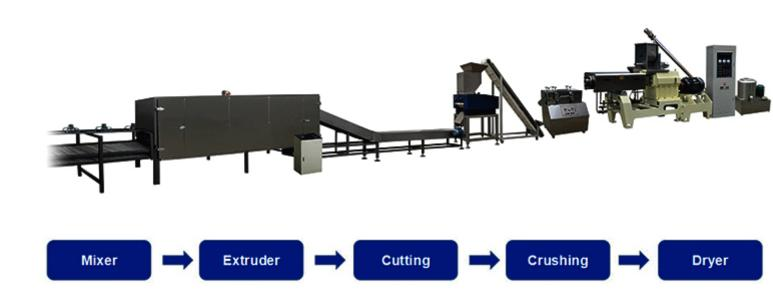
Functions of the main equipment of the bread crumb production line:
